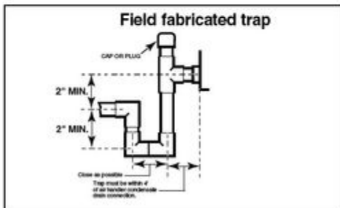
Condensate Drain Trap Example
