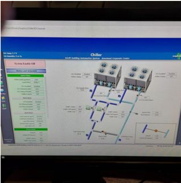
BAS Chilled Water System
